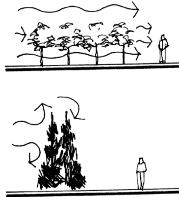
Figure 2-17. Increasing wind protection.
